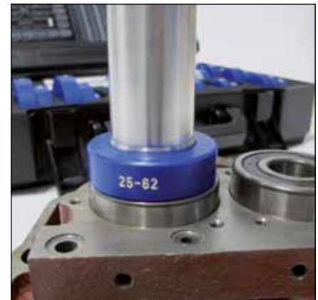
Collets are engraved and marked clearly
